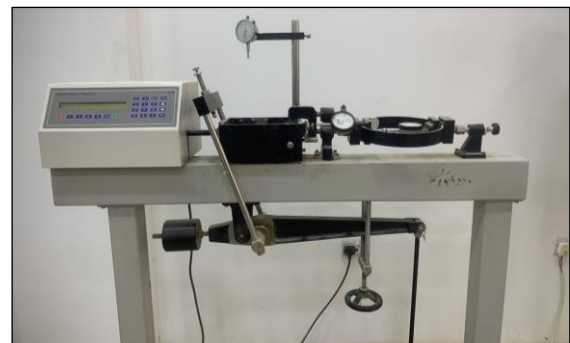
Fig. 5 The direct shear test equipment.
